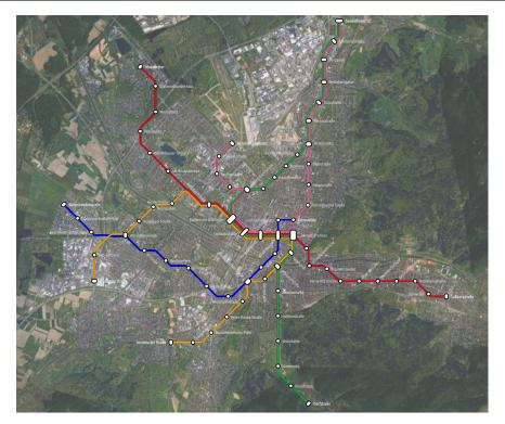
**Figure 5.45:** Octilinear map of the 2020 Freiburg tram network approximating geographical line courses, overlayed over satellite imagery.
